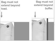
5. Buffer material should extend slightly beyond the load.
